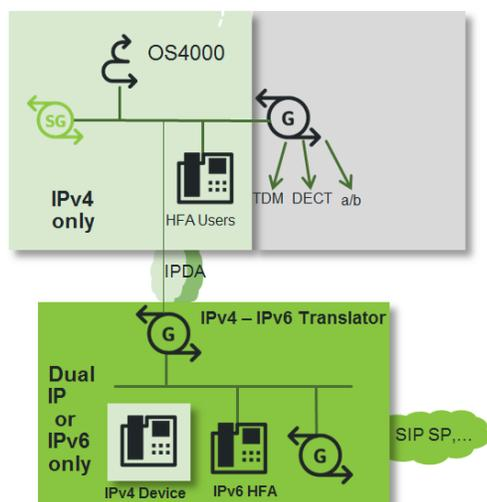
Figure: Large TDM and/or DECT oriented customer scenario, w. IPv6 branches / Devices
