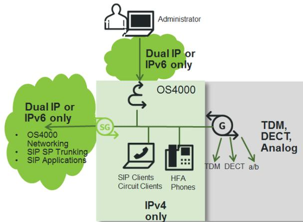
Figure: Large TDM and/or DECT oriented customer scenario w. IPv6 SIP Trunks
