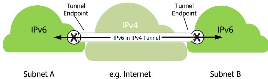
An IP-in-IP tunnel endpoint
